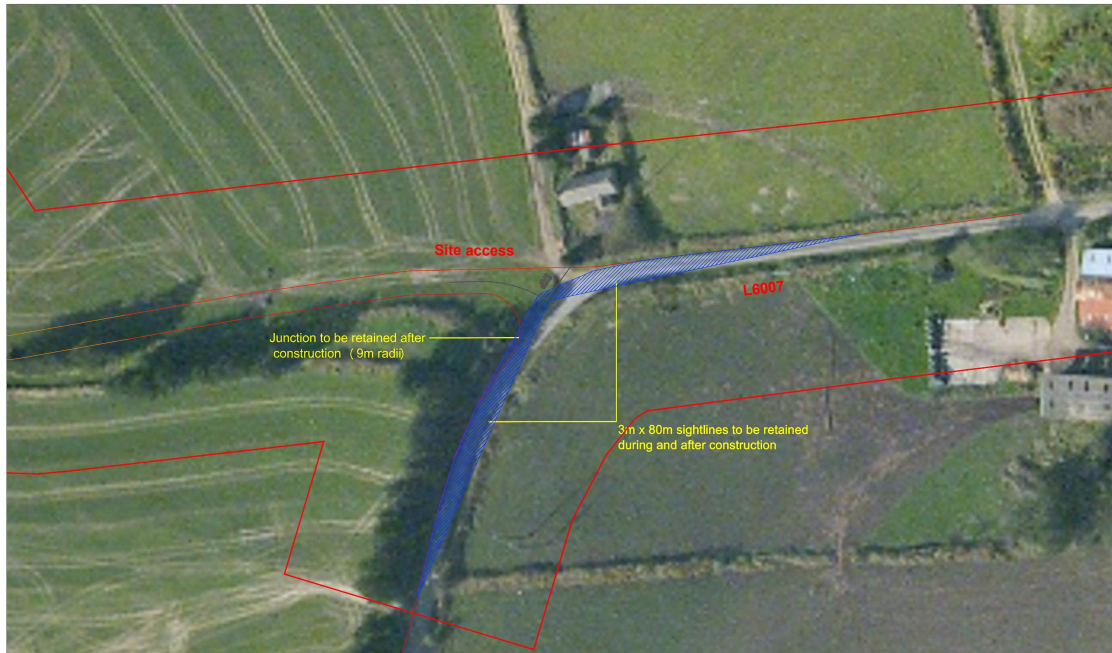
Figure 11.24 Location 10 - Access onto site off L6007, visibility splay
